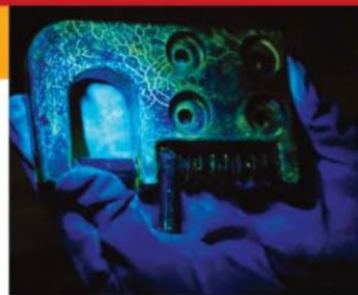
Fluorescent dye makes the cracks in this metal glow under ultraviolet light.
