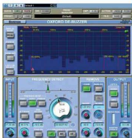
The red lines indicate problem frequencies as detected by De-Buzzer - click one to target it for hum removal
