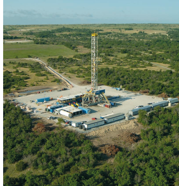
Long reach. Horizontal drilling can extend shale gas wells several kilometers from a few-hectare drill site.
