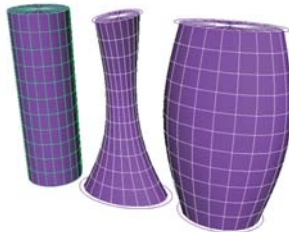
Flare: Allows you to expand or contract the top or bottom of the object.
