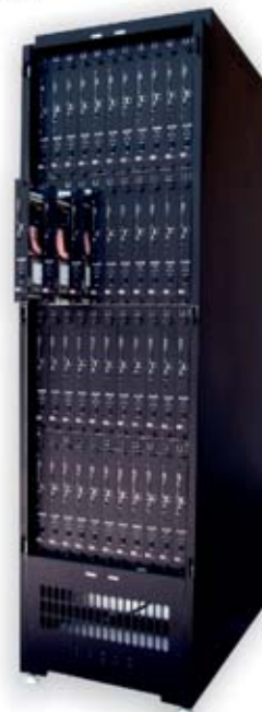
The RackSaver BladeRack Can House up to 176 Intel Xeon Processors in a Standard Rack Footprint
