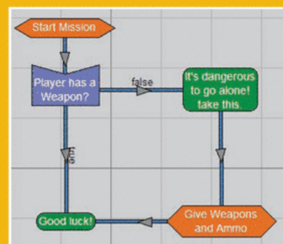
FIGURE 1 Designers create complex gameplay interactions by placing states in a graph editor and connecting states with transitions. Each state represents an action or a query and allows for logic to be created within the state graph when used in conjunction with the data in the transitions.
