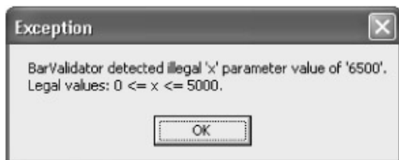
Figure 6–4: Message box displayed as a result of passing invalid value for x to the SomeObject.Bar method
