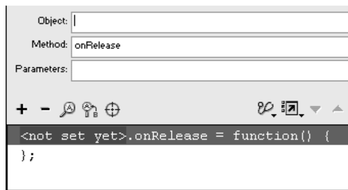
Figure 4.4. This anonymous function has yet to assign the onRelease event to a button.
