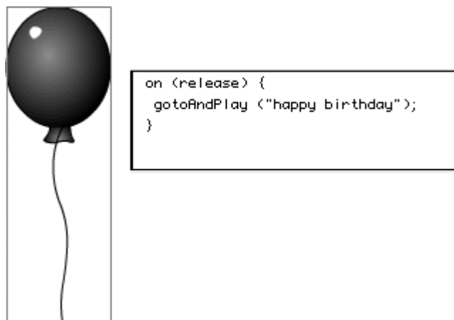
Figure 4.18. The action attached to this balloon button instance makes Flash go to the label called happy birthday and begin playing.
