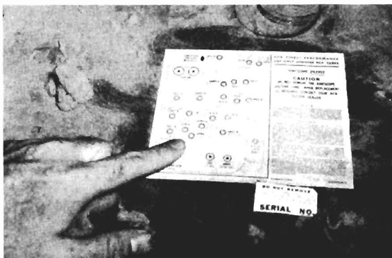
Fig. 3-1. The first move a TV repairman does is consult a component location guide that is pasted inside the case of every TV.
