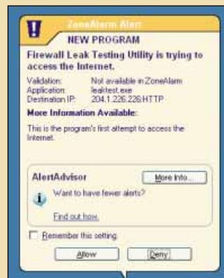
A personal software firewall improves online security, even when used in conjunction with a NAT router
