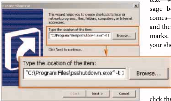
FIGURE 3: CREATE A STANDBY SHORTCUT with the free PsShutdown utility from Sysinternals.
