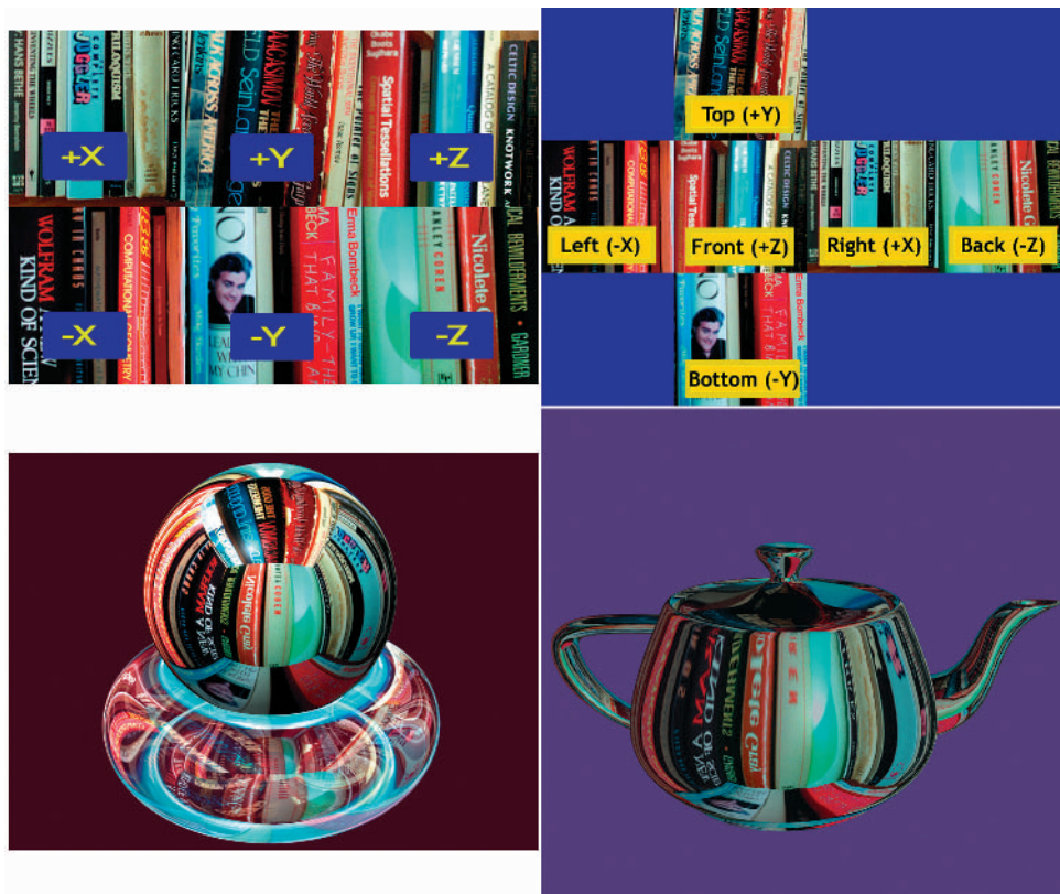
Figure 8.46 Cubic environment mapping
