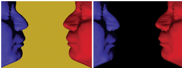
Figure 8.23 An imager shader for filling non-rendered background pixels
