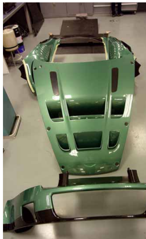
Carbon fibre composite panels laid out ready for use – only the roof of the DBR9 is still made from aluminium
