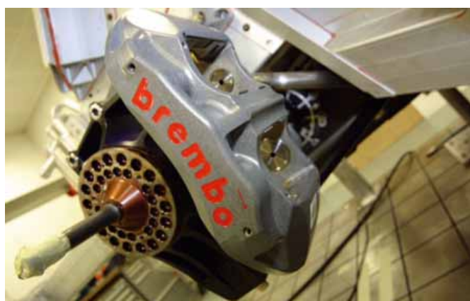
Six pot calipers and carbon discs as standard, though a steel option is offered
