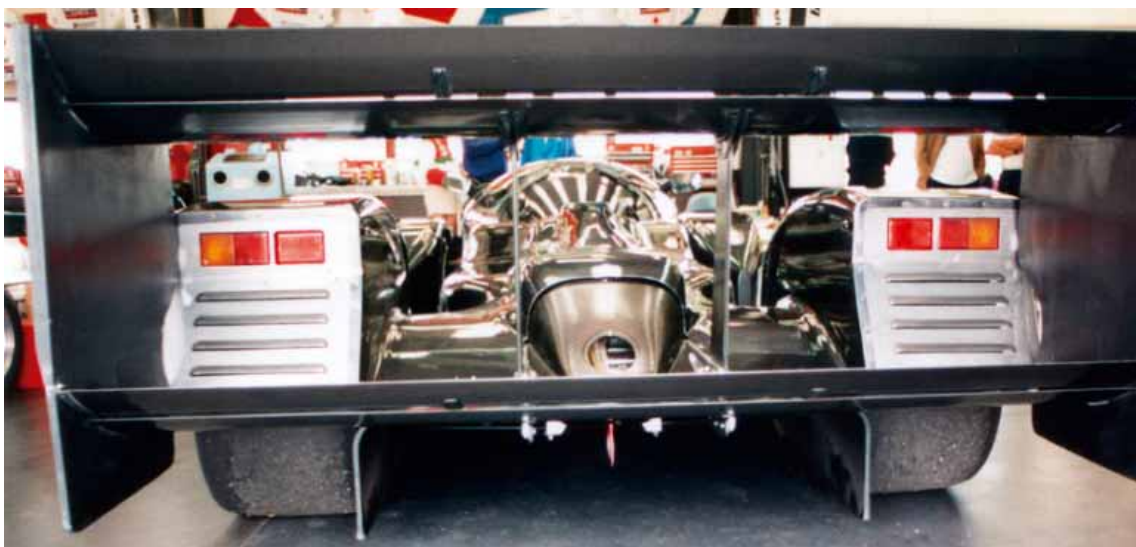
Twin-tier rear wing allowed adjustments to be made to front/rear aerodynamic balance and also to frontal downforce
