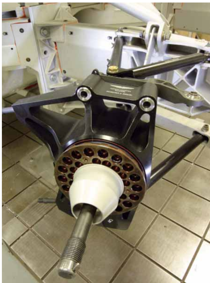
Double wishbone suspension all round uses proven Koni 2812 series dampers
