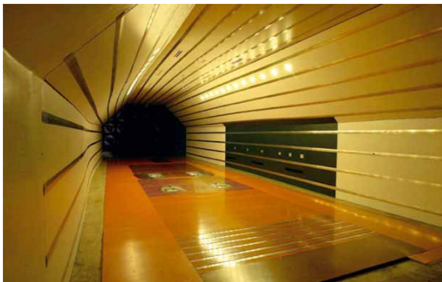
Above: internal tunnel dimensions have been honed to perfectly suit the shape of the NASCAR racecars Below: four individual rollers support unsprung weight only and spin the wheels at 130mph, while the vehicle chassis is firmly attached to four hydraulic rams. Perforations prevent boundary layer build-up
