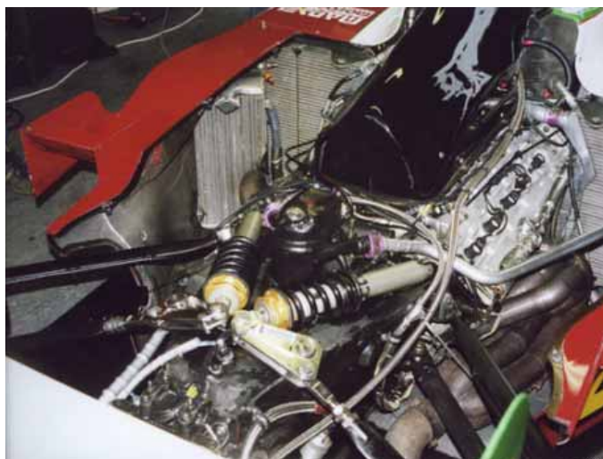
Rear suspension pickups had to be re-engineered to fit the relocated gearbox
