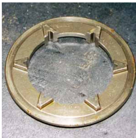
Gearbox gear dogs needed re-machining to cope with the Judd's phenomenal torque characteristics
