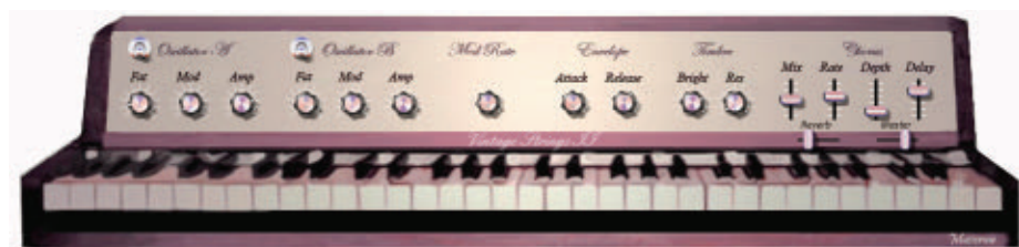
A SIMPLE PLAN > Vintage Strings MKII's spare interface sticks to common standards of retro string synths, including the simple oscillator sections and the 2-stage attack/release amp envelope.
