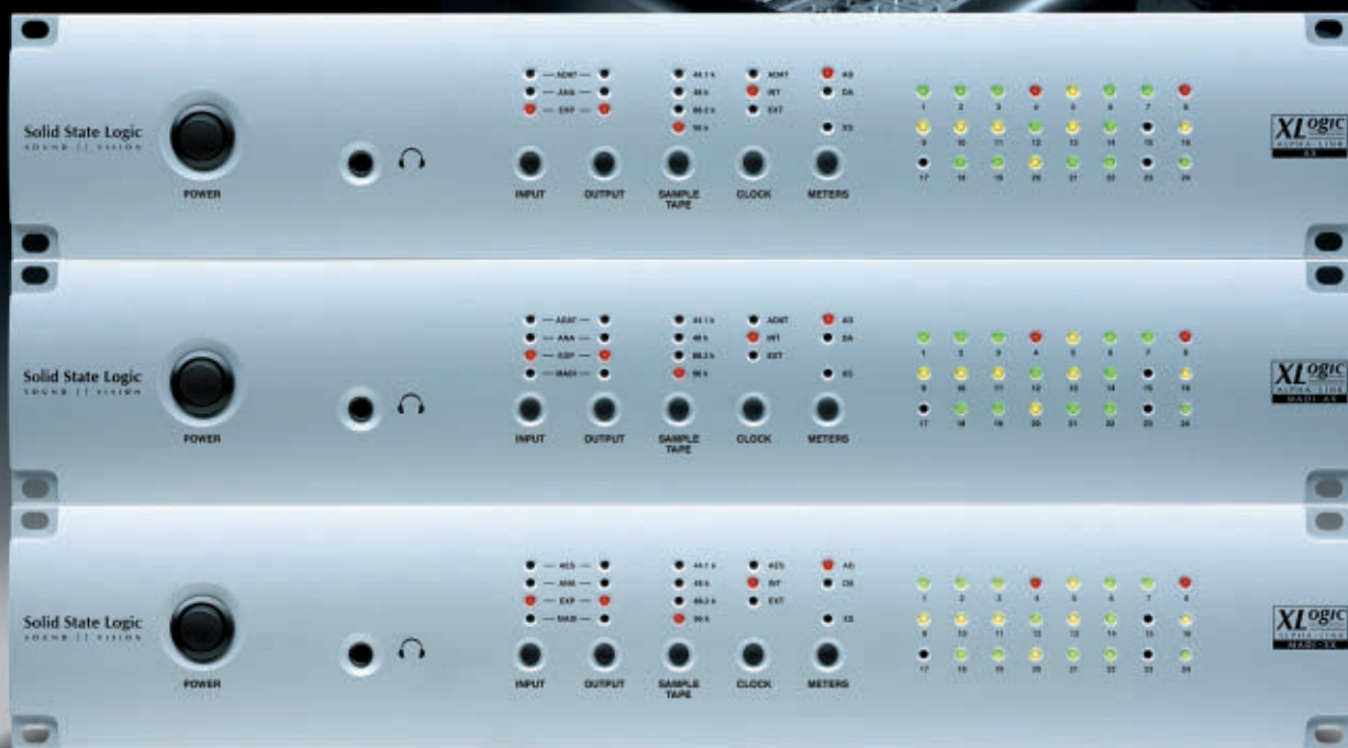
• Alpha-Link AX (top): ADAT ↔ Analogue • Alpha-Link MADI AX (centre): MADI ↔ ADAT ↔ Analogue • Alpha-Link MADI SX (bottom): MADI ↔ AES/EBU ↔ Analogue
