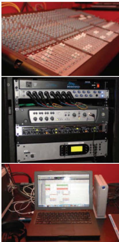
LiVE's signal flow, from top: the Mackie Onyx 80 Series console, the rack/interfaces/live-to-air streaming box and then to the mobile Pro Tools LE Mac recording setup.
