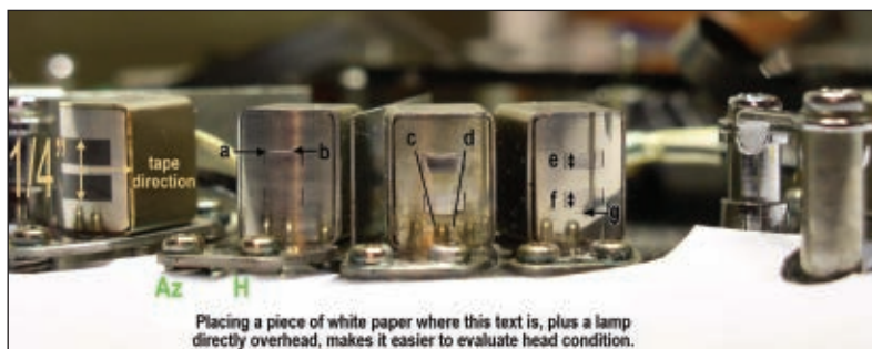
Figure 1: Four of the six heads used by the RE-301. The tape moves from left to right, starting with the erase and record, followed by two playback heads.
