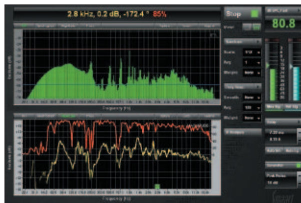
Smaart's two-up screen allows for any combination of RTA, spectrograph, magnitude or phase displays. RTA (top) and magnitude are shown.
