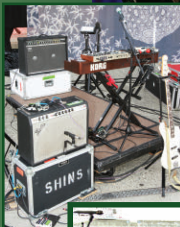
Keyboardist Marty Crandall plays the original model Korg CX-3 organ and a Korg Micro-Korg. According to guitar/keyboard tech Zivich, both boards go through Boss delays and are summed into a simplified Behringer mixer. Crandall sings through a Beta 58 as it picks up a lower level of some of his hand percussion.
