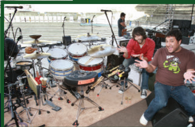
According to drum tech Davey Brozowski (above, left), drummer Jesse Sandoval's (left) kit is miked with Shure Beta 91 (kick) and 57 (snare top), beyerdynamic M88 (kick) and Opus 88 (rack toms), and Sennheiser 604 (snare bottom, floor tom). "I like Audix mics on the brass because you can heavily filter them and still retain some body—and the natural dip at 8k is also really nice," Brozowski says. "We're using the SCX-25s on the overheads. They are very sensitive mics, and if Jesse was a basher, I doubt I'd be able to use them. We use the M1245 under the bell of the ride cymbal and a Shure KSM model mic for the hi-hat."
