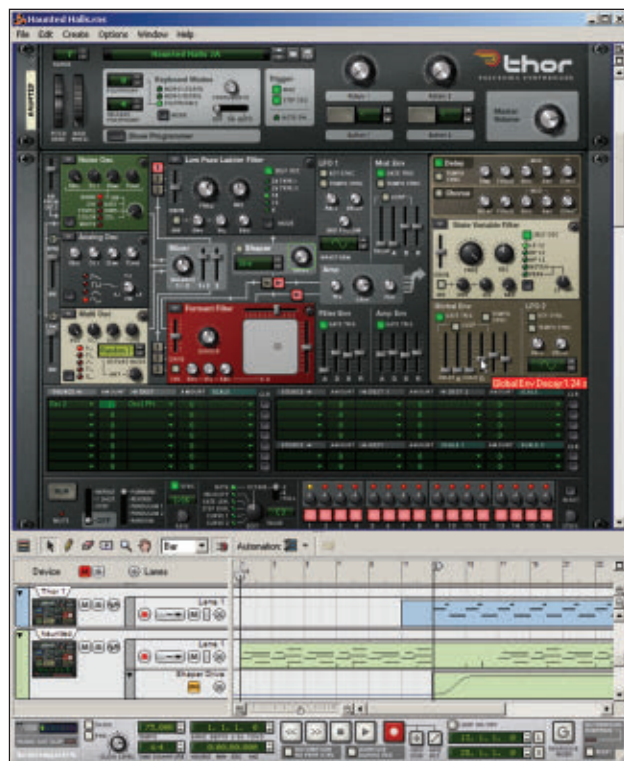
Thor boasts multiple oscillator and filter types, a deep modulation matrix and a step sequencer. The main sequencer is visible in the lower pane.
