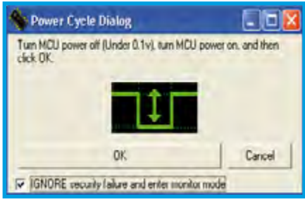
Figure 9. When the 'Power Cycle Dialog' window appears the supply voltage must be switched off and on again briefly.
