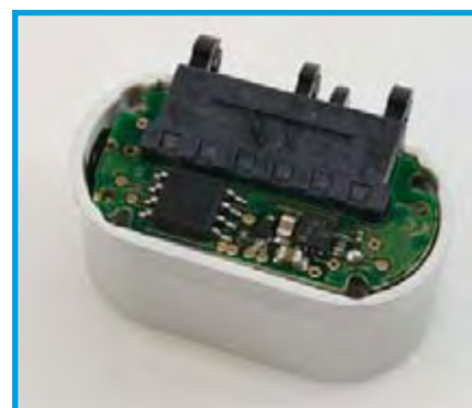
Figure 3. The step-up transformer can be seen among the passive SMD components.
