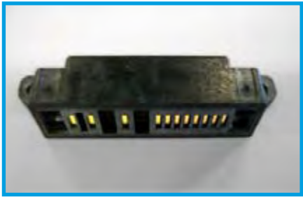
Figure 6. Programming is carried out via this connector on the phone flash. The matching connector illustrated can be bought online.
