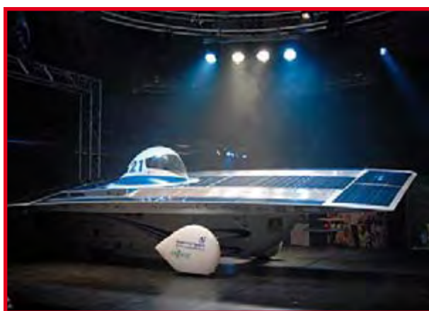
The Twente One with tilting solar panels
