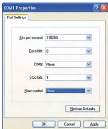
Figure 2. The settings shown here must be used for serial communication.
