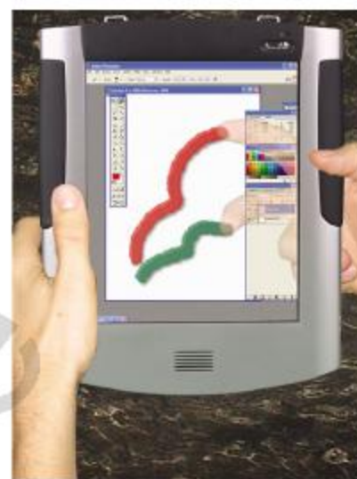
An early design drawing of LucidTouch shows how a user will be able to utilize multitouch and interact with a program from behind the screen.
